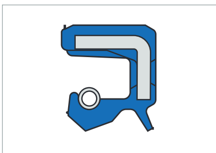
Fig. 2 Simmerring BA...SL NBR
